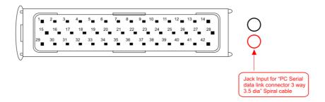
The ECU comes with a spiral cable ending with a Jack on one side and alternatively a DB9 female or a DB25 female on the other side. The Jack input of the ECU to be used is shown here above. The spiral cable is used to program the ECU as well as to communicate with external devices, like AIM ones.
