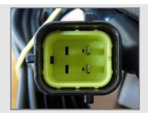
Mercury 849849 AXX interface cable has four not cabled wires you can connect to AiM devices.
