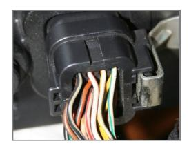
To connect AiM devices to Ducati ECU through the dashboard use its 26 pins rear connector. Here below are its pinout and the connection table.
