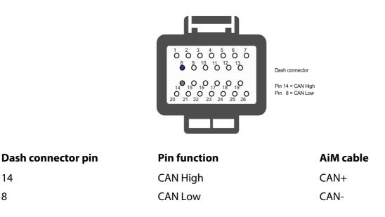
This is a slow CAN bus (125 kb/s); when connecting your AiM device to the bike you need to remove the 120 Ohm resistor that is mounted between CAN+ and CAN- in AiM device CAN cable. In case the resistor is integrated in AiM device, like is in most AiM dash loggers, then connect AiM CAN- to a GND line on pin 22 of the dash connector.
