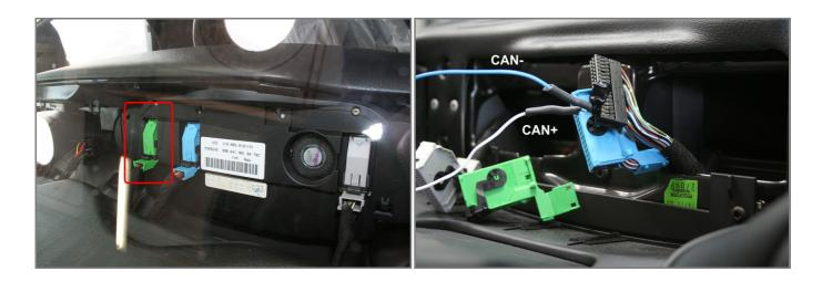
The dashboard connector is an AMP 32 pins female and, as you can see in the images here below, pins number are indicated.
