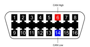
**OBDII connector pin**
